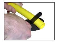
If using ID chamfer tool with gauge, check for proper chamfer by inserting pipe on gauge up to the oring. With proper chamfer, oring will begin to enter pipe.
